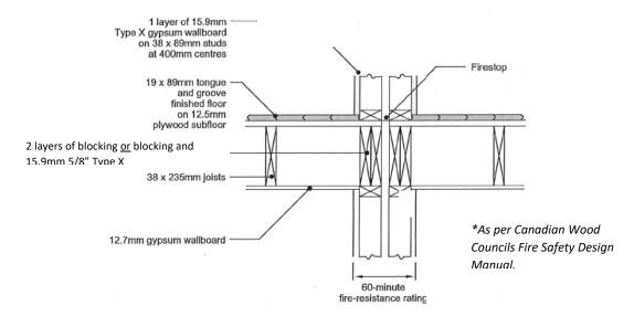
Note: The two layers of blocking are required when joists are parallel or perpendicular to the wall.
